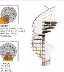
If the first tread from the bottom is not accessible, try (if possible) moving the landing point, or inverting the direction of rotation, or adding or removing rises.
