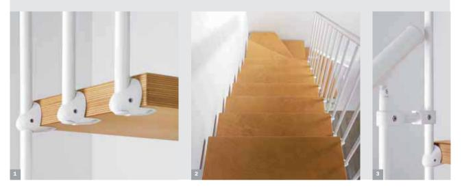
**Magia**90 can be adjusted in height, going and rotation during installation. This allows fully adapting it to the stairwell as well as choosing the configuration: rectilinear, with one curve or with two curves. The treads are in light or cherry-stained birch plywood. The handrail is in PVC with an aluminium core and is available in white or iron grey to match the colour of the staircase.
